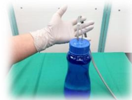
Distilled water reservoir
